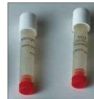
FIGURE 122 : TUBES PASSIFS POUR MESURER LES NO<sub>2</sub>
